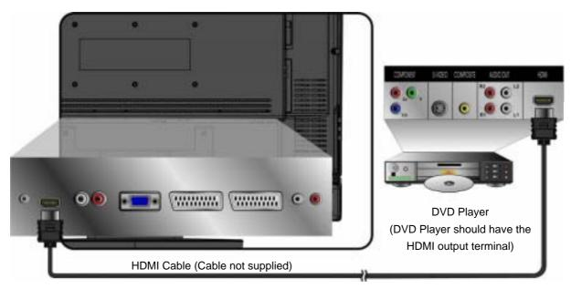
**Note:** To receive the sound from DVD, please turn on Sound Menu of OSD for selecting HDMI audio to HDMI. However, the input source should be in HDMI.
